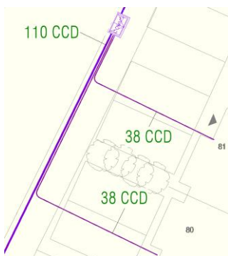
Figure 2 CCD run out from in ground chamber (JB4 or similar) to dwelling. It shall terminate in an ETU interface module prior to entering the dwelling. 110 denotes 110mm diameter in ground duct. 38 denotes 38mm diameter in ground duct.
